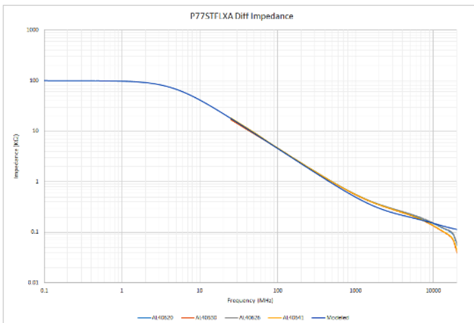
P77STFLXA differential impedance
